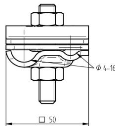
Universal clamp / earth connection clamp in bare steel for Ø 4 - 16mm / 30x3.5mm or Ø10mm
